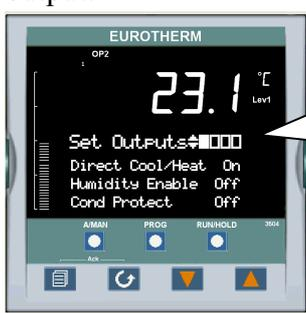
The Outputs can be switched on and off with the Up-Down Buttons and Enter to move on to the next Output
